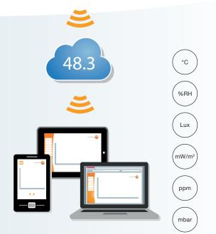
The monitoring system testo 160 monitors ambient conditions in display cases, exhibition rooms and depots. The loggers transfer measurement values by wireless LAN to the online store (Testo Cloud).
