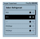
9.2 Setting the refrigerant: Press [▲] or [▼] to select the refrigerant and press [Menu/Enter] to confirm.
