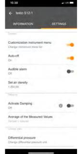
Changes to the measuring instrument settings in the app are transferred directly to the measuring instrument. Synchronization with the app is confirmed on the measuring instrument via "SYNC DONE".
