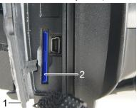
> To remove the memory card: press the memory card to release the lock.
