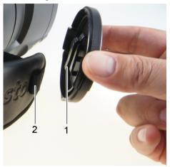
> Guide the clip on the lens cover (1) through the loop on the handle (2).
