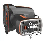
Push the battery all the way into the rechargeable battery slot until this is flush with the bottom of the handle.
