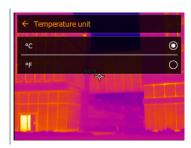
▶ The activated temperature unit is marked with a dot (●).
