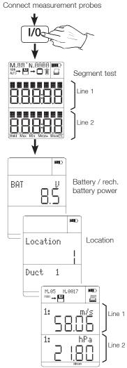
Current readings - different, depending on probe(s) connected.
