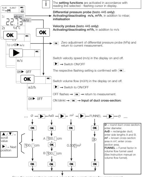
Once the cross-section is entered, return to the current volume flow measurement.
