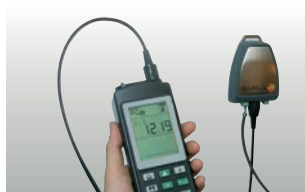
Inspection of transmitters with 4 to 20 mA interface
